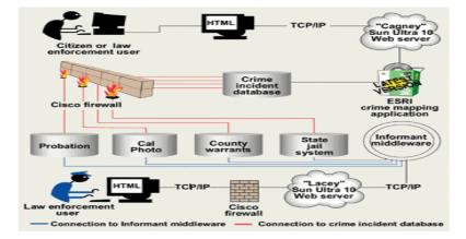
ARJIS runs on a Sun Microsystems Ultra 10 server with a 440-MHz Ultra Sparc processor. ARJIS utilizes INFOTECH, a component of a larger program called the Advance Generation of Interoperability for Law Enforcement (AGILE). The user interface is a commercial off-theshelf (COTS) Web browser, allowing officers using wireless laptops and hand-held personal data assistants, to query the databases.
